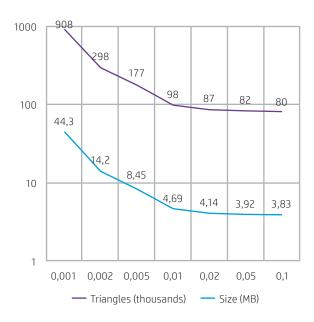
Figure 2. Triangle counts and file sizes vs. exported accuracy
